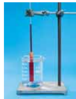
Figure 1.11 Water enters the Visking tubing 'sausage' by osmosis. This causes the level of liquid in the capillary tube to rise. In the photograph, the contents of the Visking tubing have had a red dye added to make it easier to see the movement of the liquid.
