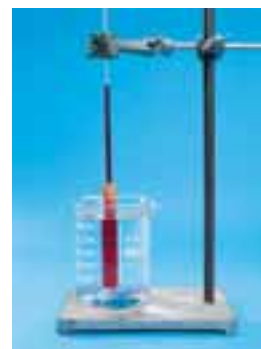
Figure 1.11 Water enters the Visking tubing 'sausage' by osmosis. This causes the level of liquid in the capillary tube to rise. In the photograph, the contents of the Visking tubing have had a red dye added to make it easier to see the movement of the liquid.
