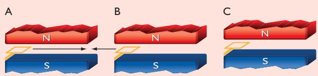
In **A** the coil is moving horizontally at constant speed between the two magnets.
