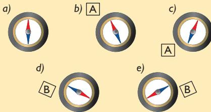
An unknown object **A** is brought near to the compass and the compass deflects towards it as shown in b) and c). A second unknown object **B** is brought close to the compass and it responds as shown in d) and e). What does this tell you about objects **A** and **B**?
