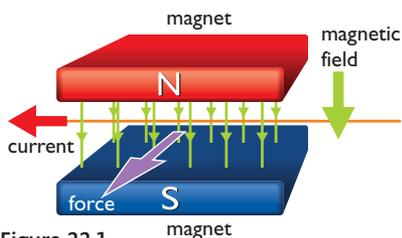
Figure 22.1 shows part of a wire carrying a current placed in the magnetic field produced by two strong magnets.
