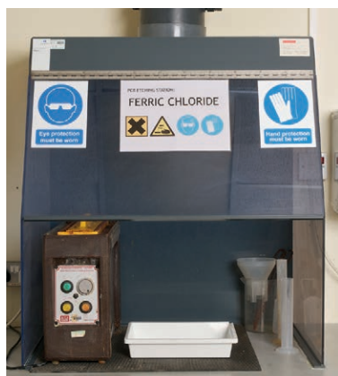
Figure 1.04 A fume cupboard used to extract potentially harmful fumes and gases
