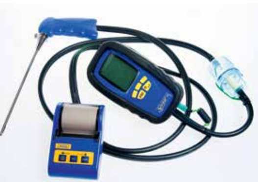
Figure 7.38 Combustion analyser with infra-red printer and flue sampling probe
