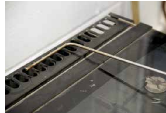
Figure 7.46 Sampling a built-in oven grill
