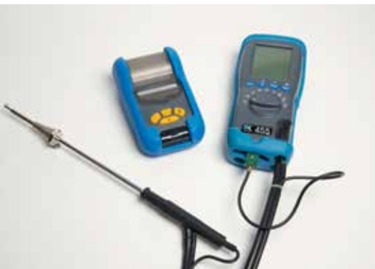
Figure 7.44 Standard sampling probe with moisture/filter protection
