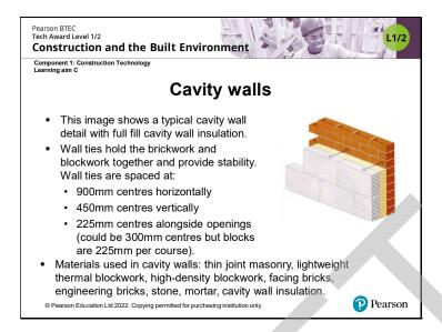
Use this slide to explain cavity wall construction.
