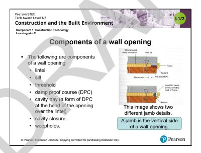
Use this slide and the next to explain the components of a wall opening. The image shows the cross-section detail through two different jambs of openings, explain how continuity of insulation is achieved and how potential damp transfer is dealt with at the point of cavity closure.
