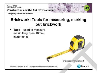
Explain that this is a standard tape measure available t=in various lengths A ruler isn't used in brickwork any more.
