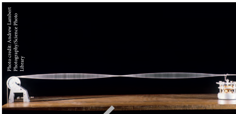
► Figure 1.52: Stationary waves in a stretched string can be demonstrated with a vibration generator, a pulley and weights to adjust the tension
